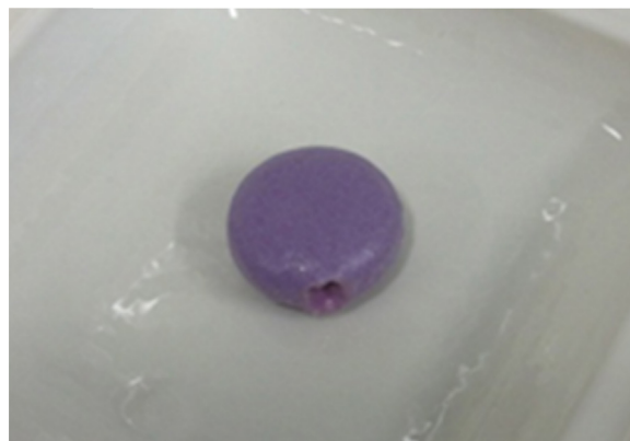
Fig. 1. Visible rupturing of enteric coating after storage at 40^\circ\text{C} ; 75% RH for eight days.
