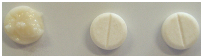
Fig. 3. Sodium valproate tablets after 21 days of storage at accelerated (left), refrigerated (middle) and controlled room temperature (right) conditions.
